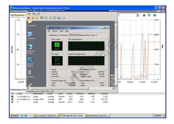
An administrator has deployed a new virtual machine on an ESXi 5.x host. Users are complaining of poor performance on the application running on the virtual machine. Performance tools display the results shown in the exhibit.
