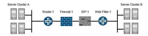
You need to filter east-west Web traffic inside the data center between Server Cluster A and Server Cluster B using information contained in the IP header. Referring to the exhibit, where should you filter the traffic?
