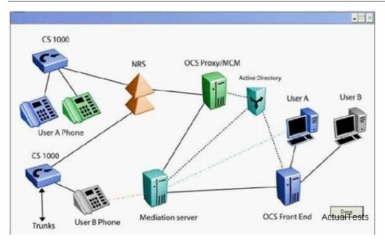
You have been asked to troubleshoot a Nortel Converged Office solution for a Communication Server (CS) 1000 Rls. 5.0 network. The customer requirements include a centralized numbering plan arrangement using SIP Trunking. Click on the component in the diagram that is required as part of the centralized numbering plan for the network.
