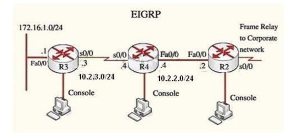
Presently JS has configured EIGRP on all routers in the network R2, R3, and R4. Your duty is to find and solve the connectivity failure problem with the remote office router R3. You should then configure route summarization only to the distant office router R3 to complete the task after the problem has been solved. The success of pings from R4 to the R3 LAN interface proves that the fault has been corrected and the R3 IP routing table only contains two 10.0.0.0 subnets.
