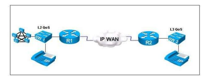
Traffic flows from the IP phone that is connected to SW1 to the IP phone on SW2. If the trust boundary has been extended to the IP phone on SW1, in what two places will traffic be marked and classified so that the proper QoS settings may be carried through the network? (Choose two.)
